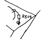
push the loop onto the feedthrough using the tip of a screwdriver blade (the loop should be tight enough to hold the resistor in place as you solder it), solder the feedthrough connection, and connect and solder the other end of the 100 ohm resistor at the bandswitch waffer lug.
